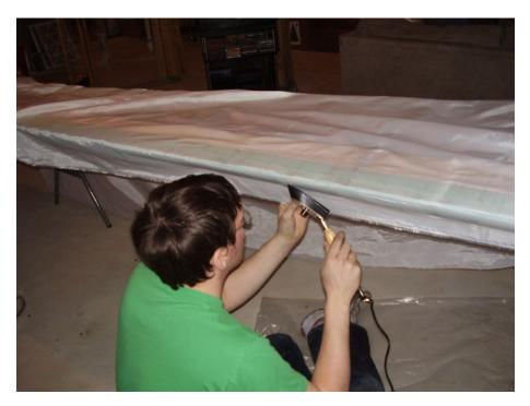
We glued three inches either side of the leading edge and along the root and tip and both side of the trailing edge. The fabric laid in place pretty well. We would heat the leading edge in place first and then work the top of the leading edge in place.
