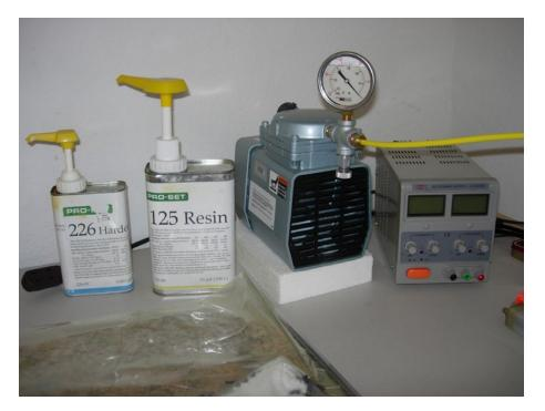
Above: Resin and hardener, vacuum pump, hot wire power supply, and vacuum bag.
