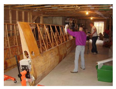
I knew the general Stewart's process from doing the control surfaces but had never covered anything nearly as big as a wing before. We started out by cleaning the wings with the heavy duty cleaner, and then painting glue around the perimeter of the
