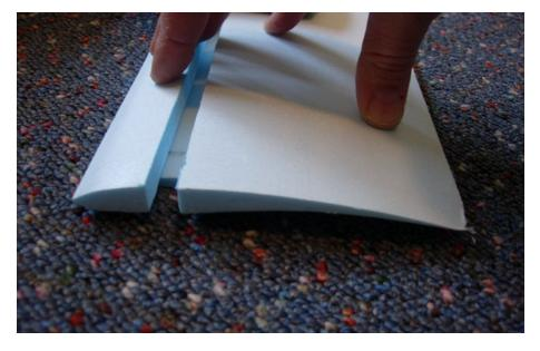
Foam core of KB18 wing panel with cutout for carbon fiber spar system. Text provides more details.
