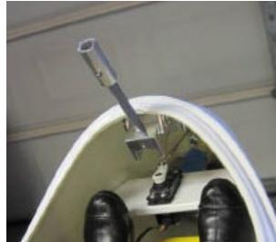
Canopy removed to show the canopy hinge in the up position. The hinge is glued to the fuselage interior with shoe Goop.
