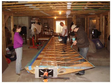
wing and along each rib. Then, with the glue somewhat dry, we laid the fabric in place over the wing and used the iron to reactivate the glue and set the position of the fabric. This worked like a dream.
