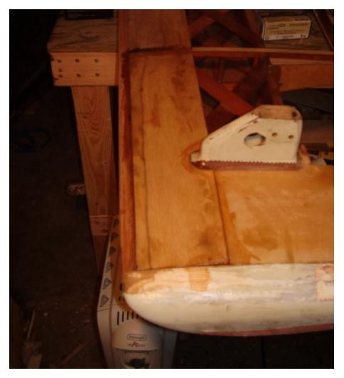
Rotten wood replaced on the bottom of the right wing.
