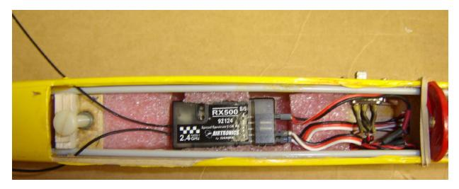
Because of the small fuselage width the receiver is mounted under the wing. I punched small holes in the sides and routed the two antenna through them. One antenna is taped to the side while the other is taped to the bottom of the wing at a 90 degree angle.
