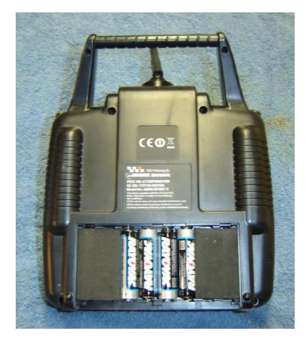
Left: The rear battery cover is removed from the transmitter and four AA size dry cells are installed. The low battery count makes the transmitter very light and easy to hold.
