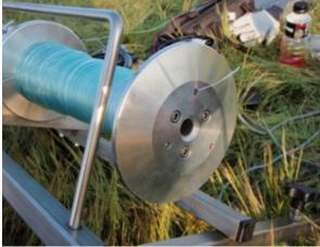
Above: Winches set up and ready to go. Left: Typical F3B winch drum - wide and with a small diameter so the motor torque pulls consistently as the line reels in. Monofilament line stretches and F3B launches can be quite spectacular.
