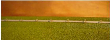
Left: End view of the KB 18 tip joimt. Above: Turbulator made from 1mm segments of 1 mm monofilament fishing line spaced at 1cm intervals.
