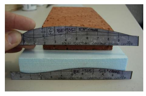
Metal templates for the root of the KB18 wing tip. BE 9051 airfoil, 5.3" chord. Spar location marked forward of 30% chord.
