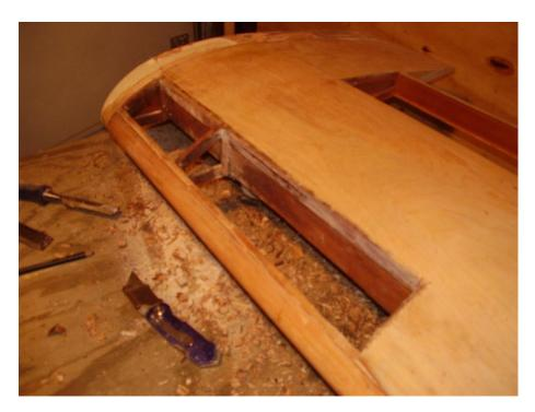
Rotten wood removed from the top surface of the right wing.
