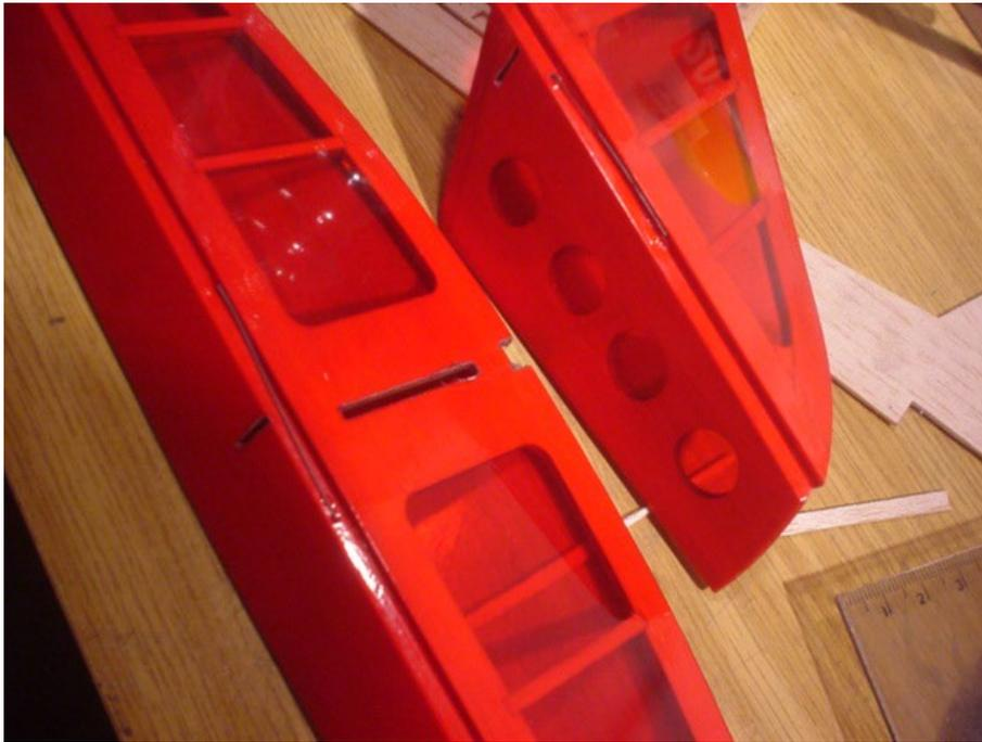
slide the tail group into the slots of the tail boom and add a few drops of thick CA.
