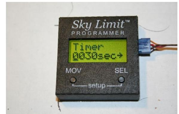
both together. For example, in an ALES contest you would set both, typically 200 M for altitude and 30 seconds of motor run time. For an F5J type contest you might only use the altitude limit. For some other LMR type events you might only use the time limit.
