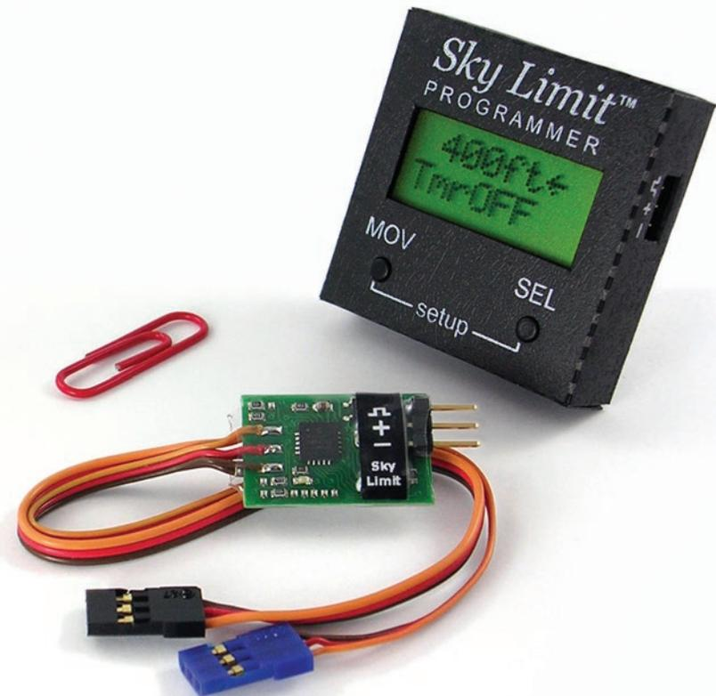
The Sky Limit consists of two separate parts, the airborne unit and a programmer. You don't need a PC to program the Sky Limit but you do need the programmer. It cannot be programmed, as some other limiters are, by moving the transmitter sticks or with a PC. However, one programmer can be used with any number of airborne units. So for example, a club could order as many airborne units as desired and just one or two programmers to share between the club members.
