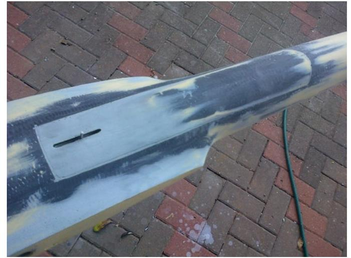
▲ *Fuselage access hatch*
