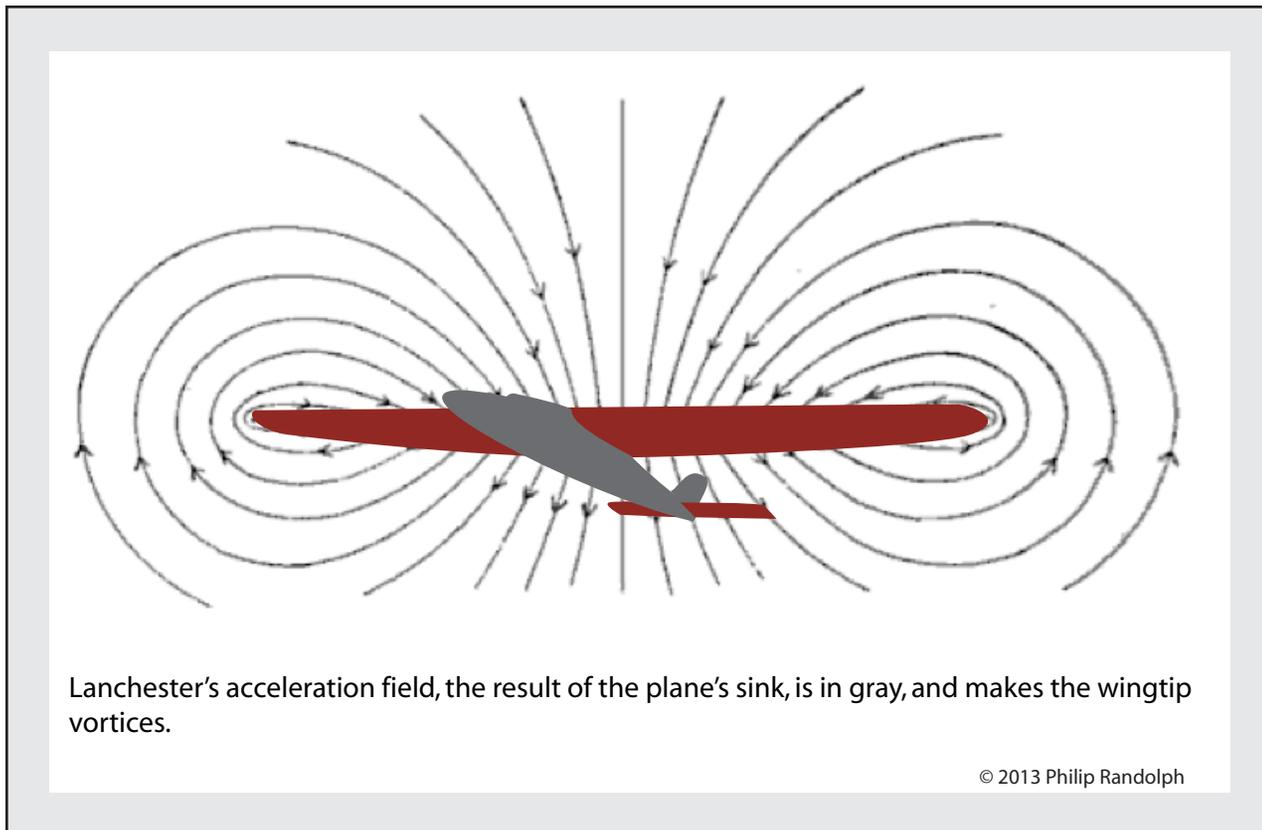
*Figure 2: Lanchester's sinking vortex. All wings fly within air that on the average, inboard of their wingtips, is sinking. Air outboard of wingtips is displaced up. All wings fly within this great swirling pattern. But its pressure and velocity profiles can be designed.*
