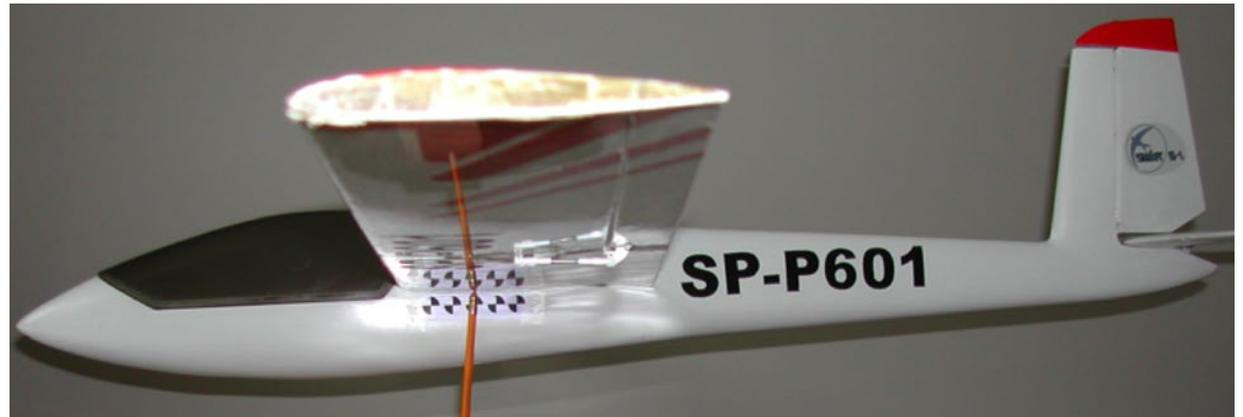
*This configuration of CGA significantly increased the longitudinal stability of my 2 meter scale Swift's small stabilizer.*
