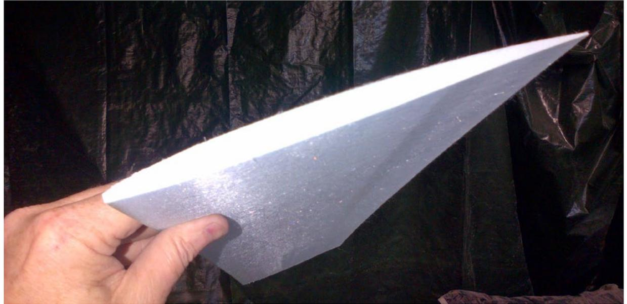
*The wing core showing the thin section used.*
