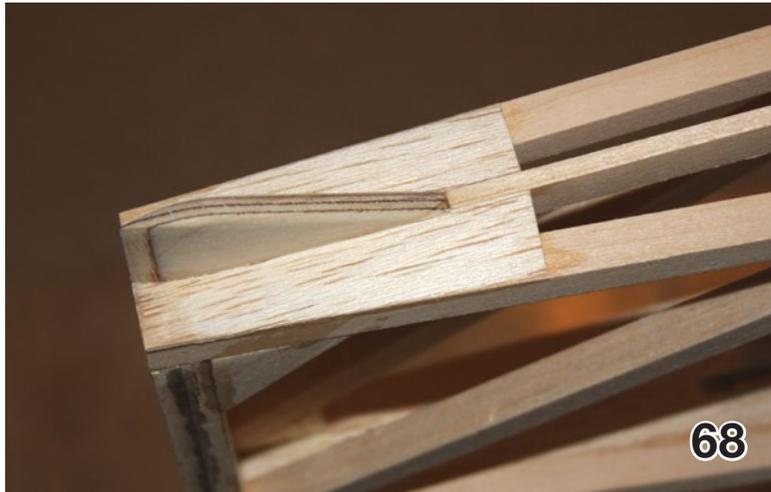
On the screw holes in the basswood blocks, I hardened the threads by applying CA into the screw holes after removing the screws.
