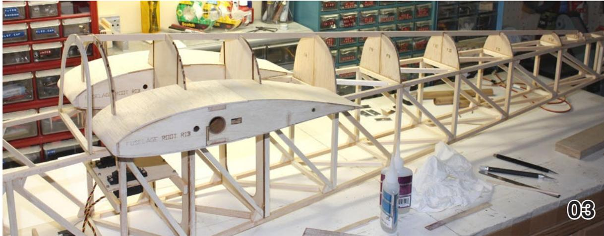
If you have a vario and plan to use a total energy (TE) probe, now is the time to install the TE tubing.
