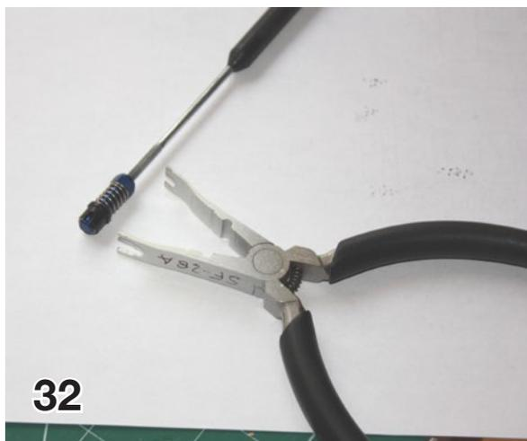
to fit around the sleeve on the Sullivan connector. You simply squeeze the pliers to compress the connector sleeve and release it from the ball. This makes it quick and easy to use inside a fuselage. See pic 32 - 33.
