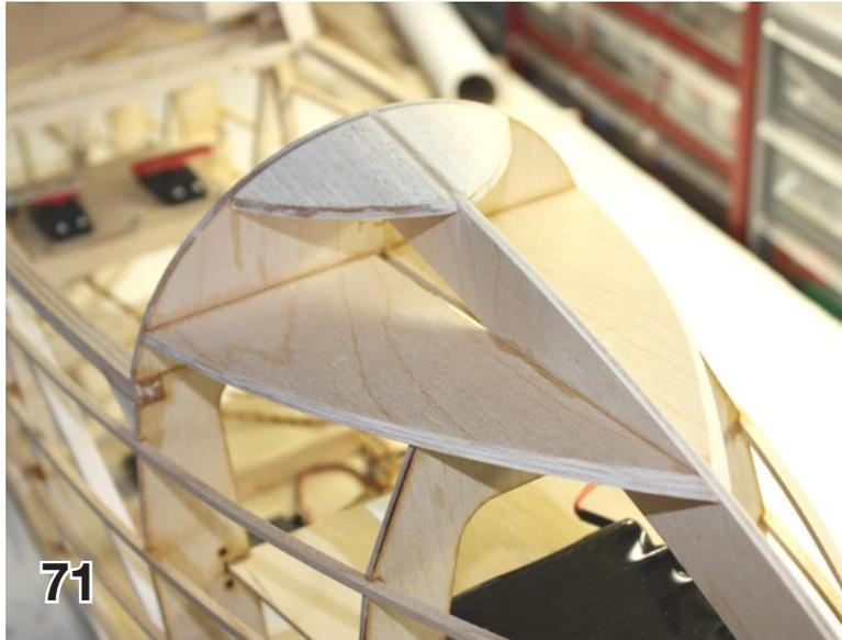
Use the plan templates to cut the 1/2" balsa contour blocks, and the 1/8" thick X 1/8" wide ply pieces that go underneath the contour blocks (to reinforce the thin edge after sanding).
