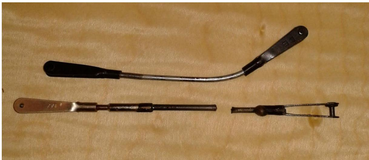
*Bent and broken clevis rods.*
