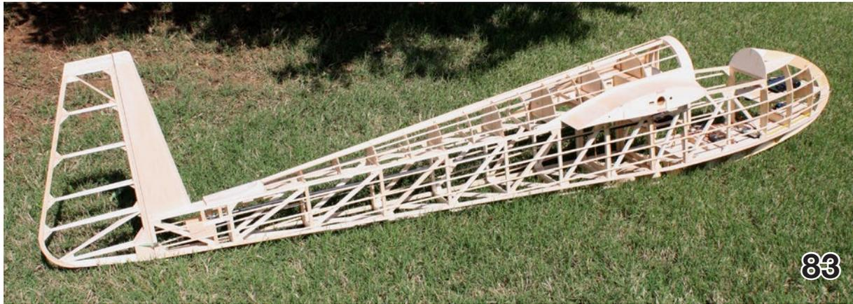
Now look at the forward ends of the nylon cable guide tubes and see if they are lined up with the cables. If not, file or sand the notches in the forward vertical member under the stab until the nylon tubes align with the cable right in the center, then CA the tubes to the vertical. See pic 82.
