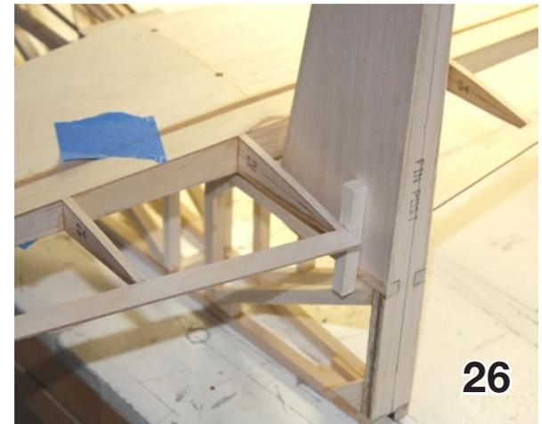
26. Stabilizer and elevator in place on the stabilizer mounting block.
