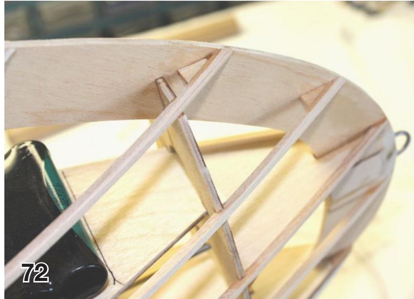
Since the fuselage covering stretches across the stringers, it cannot attach directly to the fuse longerons and still have a nice smooth shape. So 1/16" X 5/16" hard balsa strips are added to the outside of the fuse longerons and beveled so the covering will transition smoothly to the stringers.
