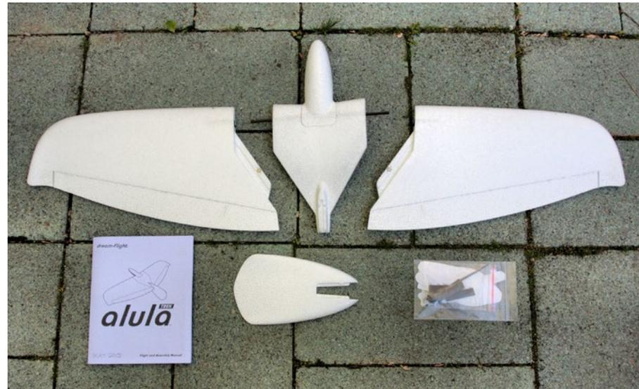
*Alula-Trek kit contents: five molded foam parts - wing halves with elevons pre-hinged, fuselage with hatch, vertical fin. Also a complete hardware bag and the superb construction, trimming, and flying manual.*
