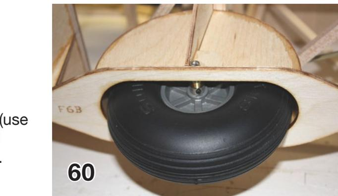
60. Wheel in place with wheel collars and brass tube spacers to maintain centering of the wheel in the well.
