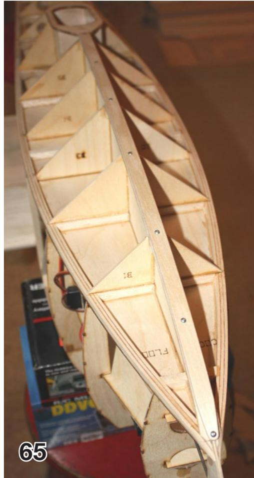
Tape or clamp the skid in place, making sure it is centered, then drill the seven holes with a 1/16" drill bit to a depth of about 5/8 inch.
