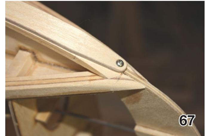
skid onto the keel using #2 X 1/2" button head screws. See pix 64 & 65.
