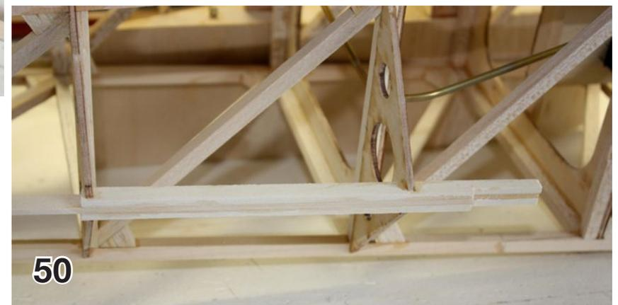
*48. Bottom formers B6 - B11 installed and bottom 1/8" x 3/8" basswood stringer installed.*
