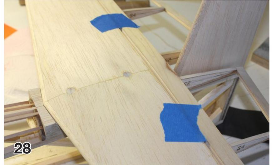
I taped a piece of brass tube onto my drill bit for an extension to drill the 1/4 holes.
