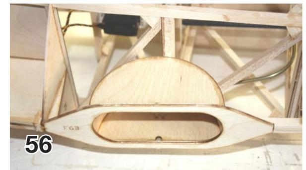
If you haven't already done so, notch out the balsa cross piece at the bottom of fuse former F6 to match the notch in F6. Fit check the wheel well, make any adjustments, and glue to the keel, bottom stringer, and F6 with CA+. See pix 55 & 56.
