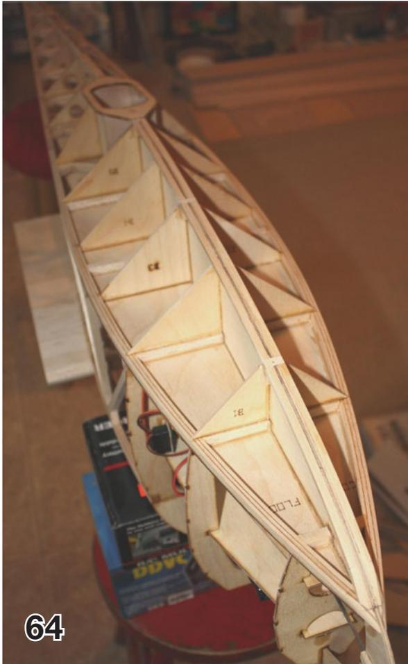
Mark the skid where the holes will be drilled. There should be one screw at each of the three blocks on the keel, one screw between each block, and one screw at the nose for a total of seven holes.
