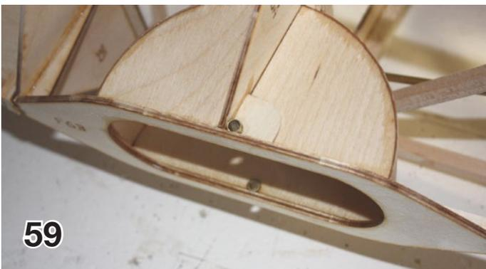
59. The 7/32 O.D. brass tube axle carriers installed.
