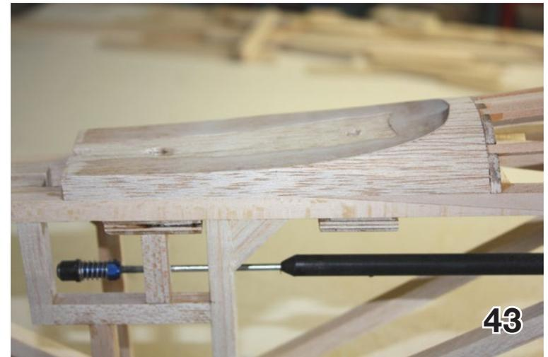
*40 - 43. Using a Monokote separator, a mixture of epoxy and microballoons is used to get the stabilizer mount to exactly fit the stabilizer.*
