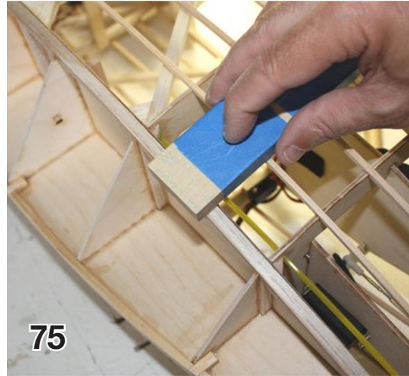
I lived dangerously and planed mine close, finishing with a sanding block, first with 100, then 220 grit.
