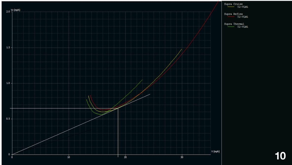
The bottom of the thermal mode curve is nice and flat, giving you a speed range from 14.5 to 16.5 mph with little penalty for deviating from the optimum at 15.5 mph. This is one of the reasons why the Supra is so easy to fly.
