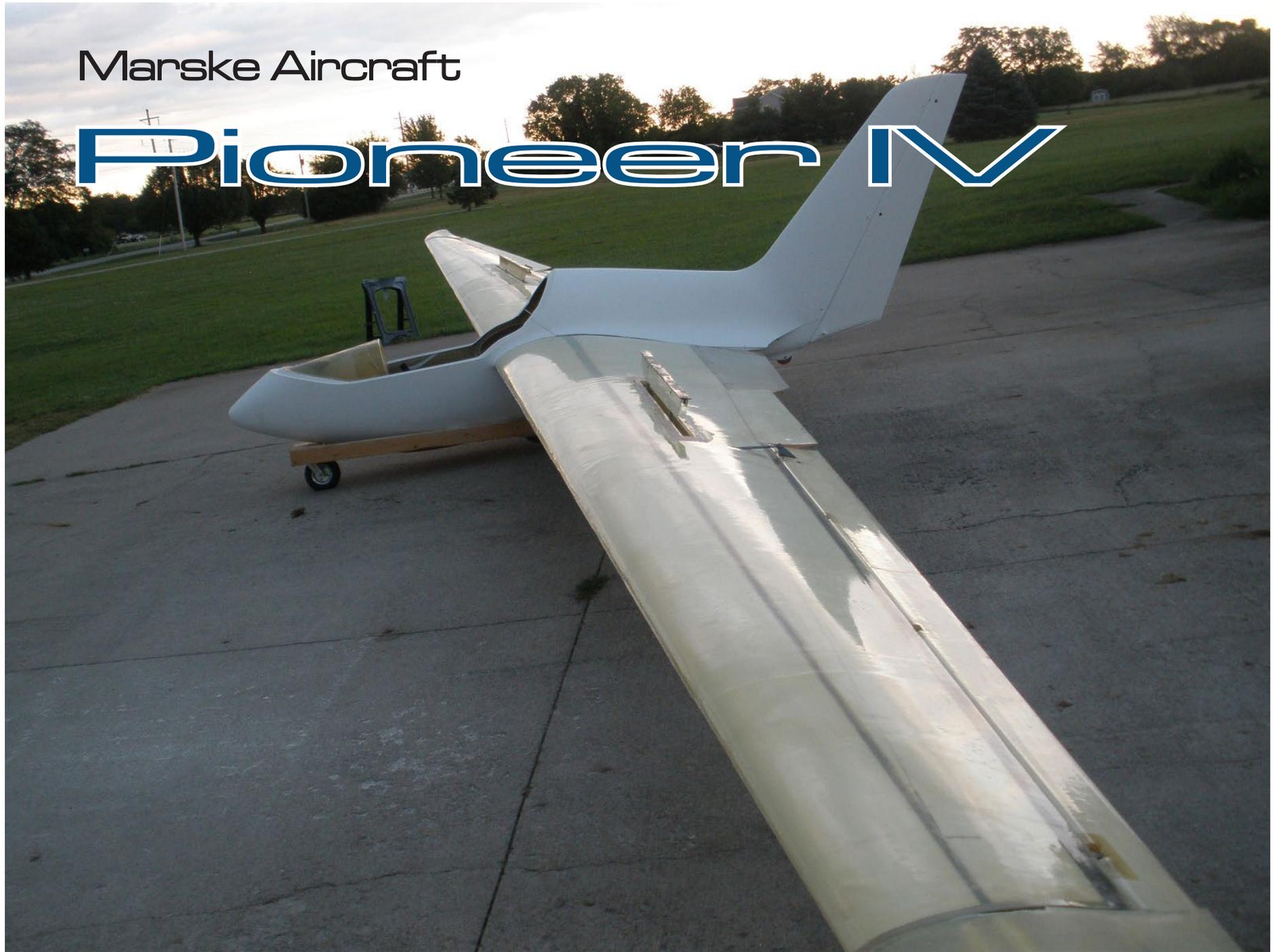
The Marske Aircraft 15 meter Pioneer IV has made a few low hops so far off the winch before winter stopped operations. It shares essentially the same planform as the Pioneer III, with only a minor change to the trailing edge contour in the area around the outer end of the central elevator. Huge differences appear in the airfoil used and the construction materials.
