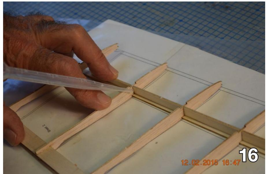
The egg-crated rib and spar can be aligned with the desired sweep before gluing with CA.
