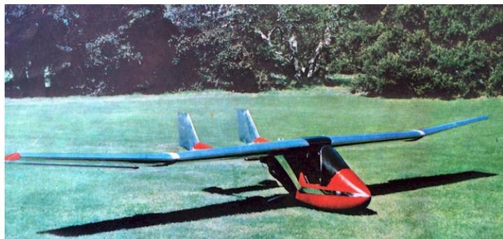
I hope they did more than just change the sweep of the T-10 wing to create that. The NACA 230 series airfoils don't have the positive pitching moment to make forward sweep work and pitch control on the outboard section of a forward swept wing generally isn't a good idea.
