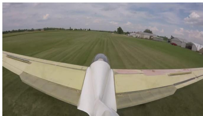
I developed a new laminar airfoil that requires a minimal amount of elevator travel over its entire speed
