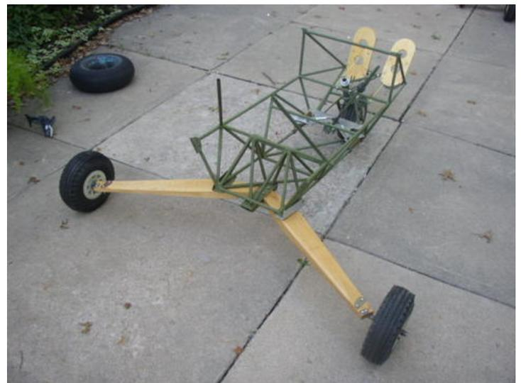
I considered it such an important deficiency that I designed a cantilever gear as shown in the photos (above). I did alternate designs, shooting for a deflection of 1-1/2" under full takeoff weight. The birch gear was lighter than aluminum or Scotchply, plus less expensive and easier to make, so that's what was used. After it was built, we loaded it to gross weight to
