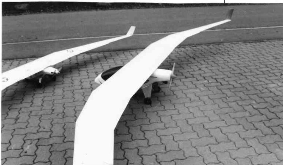
Thomas calls it a "Super-Delta" which is a pure flying wing with a high lift center, Horten type outer wings, and winglets. The cabin is a self contained sort of solar mobile, where you hang under the wing.
