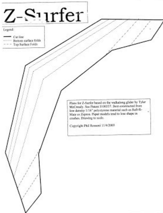
A walkalong glider is a lightweight, slow flying model aircraft designed to be kept aloft by controllable slope soaring in the rising air generated by the pilot who walks along with the glider as it flies, usually holding a paddle. Hands or even the forehead can also be used to create an updraft.
