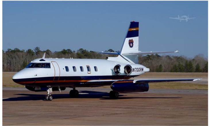
This is a Jetstar II version. Note the larger air intakes on the engines for the turbo-fans and the relocation of the bullet tank to below the wing and made more streamlined. The quirk was its lack of performance at high altitudes and shorter runways meant this version couldn't takeoff where as the turbo-jet could make it.
