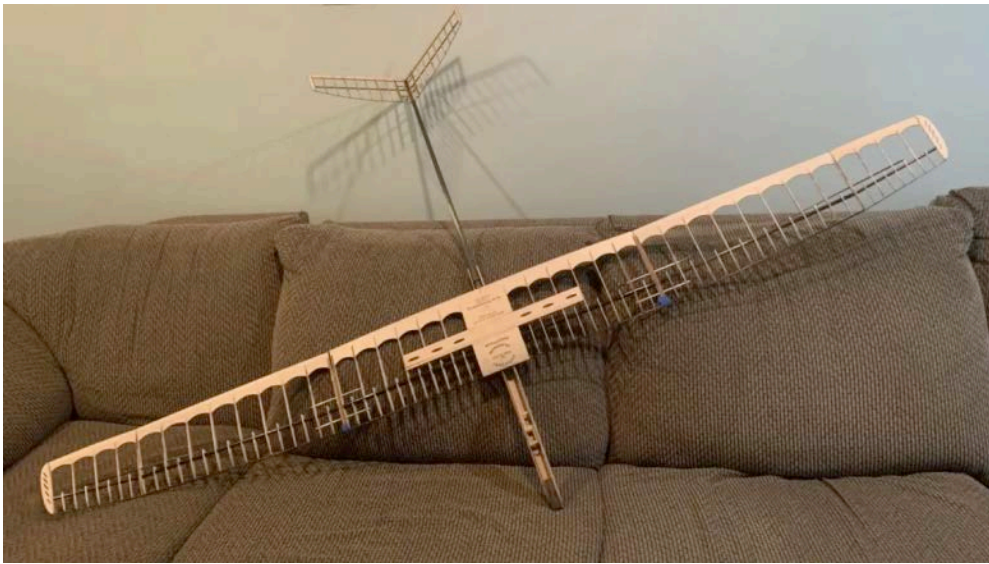
The author's Yellow Jacket 2M Competition GS under construction.
