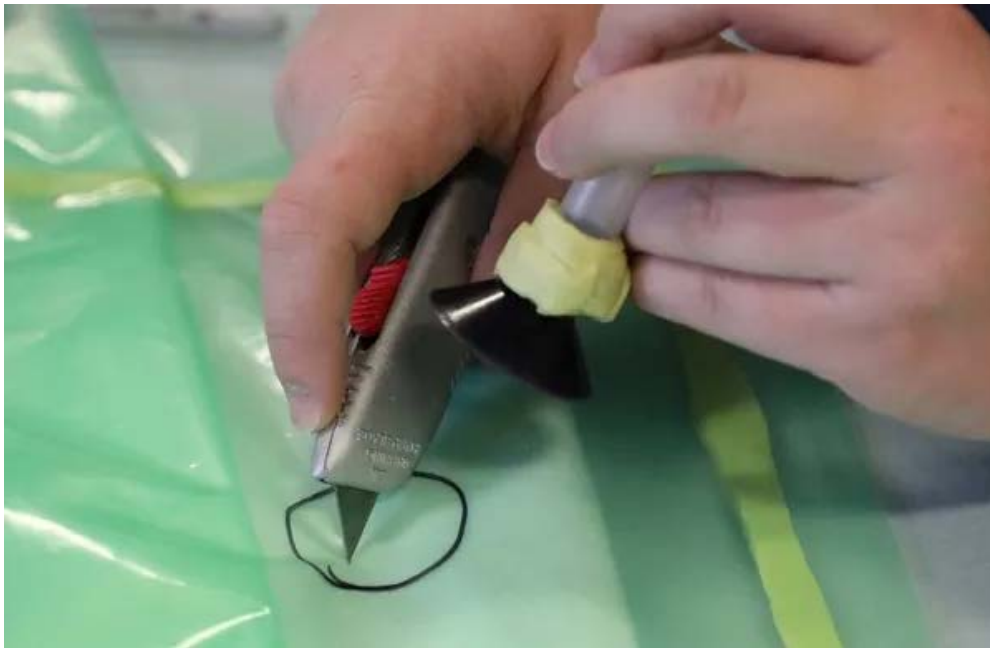
Left: The fundamentals of pleating vacuum bagging film (click for larger image). | Right: Fitting the vacuum port.
