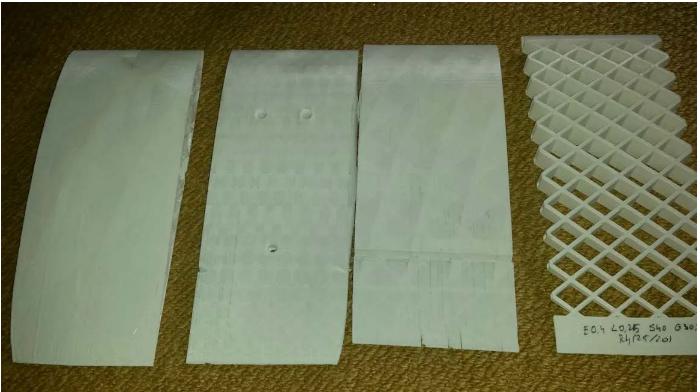
Bad prints with a small nozzle and transition to a geodetic structure.
