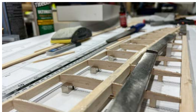
Cube magnets hold the rib stand-offs/legs square.
